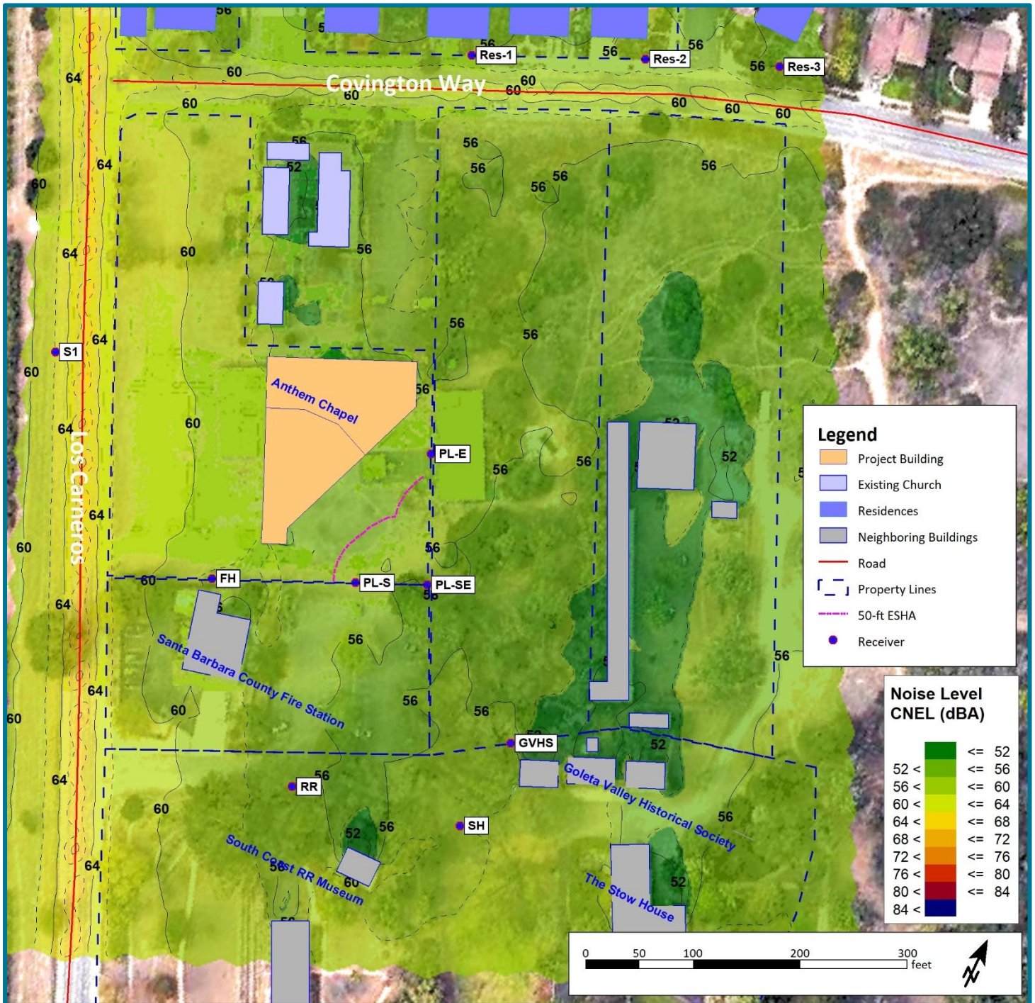
Figure 11: Ambient Sound Level Contours with Buildings in Place, Plan View
