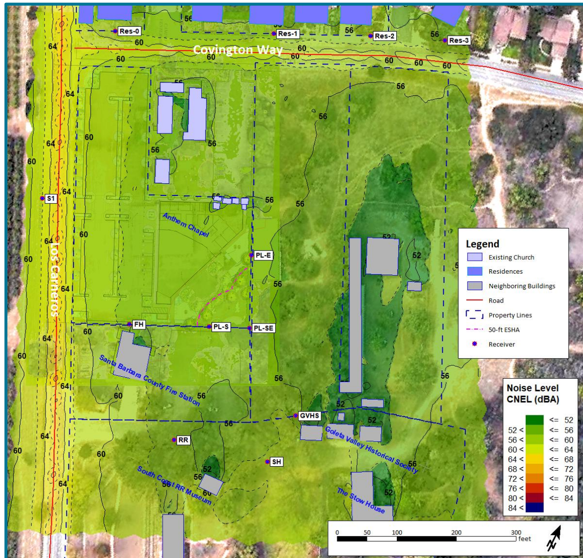
Figure 9: Existing Ambient Sound Level Contours, Plan View
